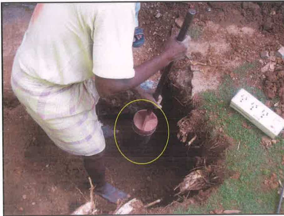
Extraction of undisturbed soil sample from founding level in progress
