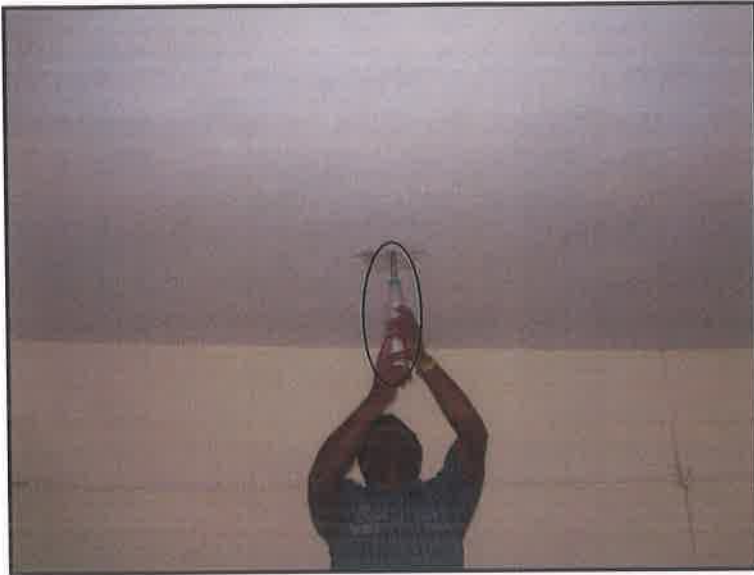
Rebound Hammer test on RC slab in progress
