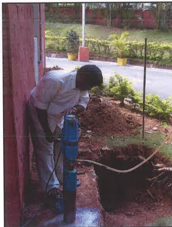
Extraction of concrete core sample from footing in progress
